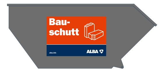
The **building rubble container** is exclusively for mineral waste such as e.g. concrete, bricks, tiles and ceramics.
